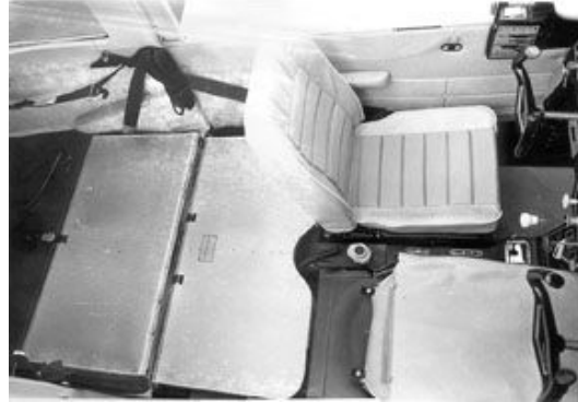
Unique among light aircraft of the era, the Tiger's rear seats fold forward, opening up the cabin for cargo space.
