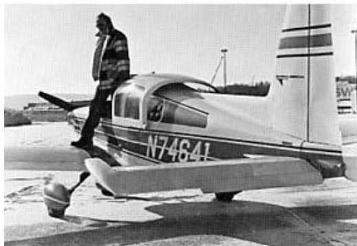
The slide-back canopy is sporty and can be opened in flight about 10 inches. It's great in summer, not so great in rain.
