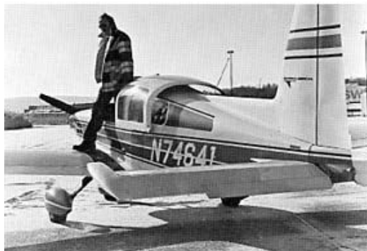
The slide-back canopy is sporty and can be opened in flight about 10 inches. It's great in summer, not so great in rain.
